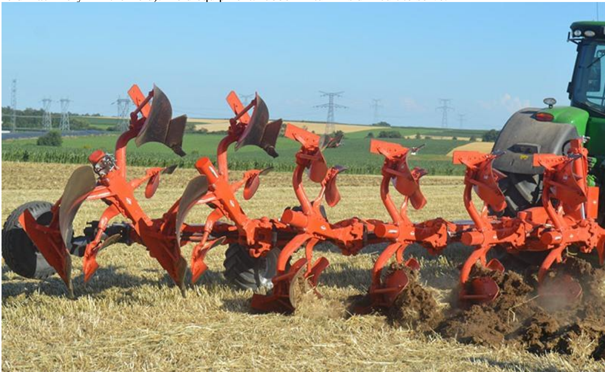
Fig. 3. Plowing by the Master L. plow firm Kuhn
