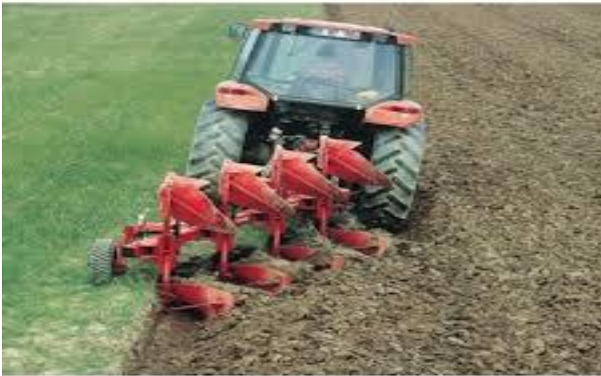
Fig. 1. Plowing with a reversible plow
