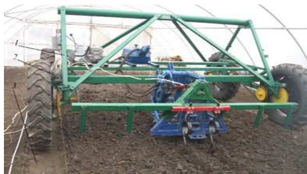
Fig. 1. The conceived and manufactured gantry tractor: 1 – frame; 2 – electric motors; 3 – permanent traffic lanes
