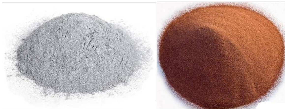
Fig. 1. Photos of sprayed powders. On the left aluminum powder A 20-11, on the right copper powder C01-11.
