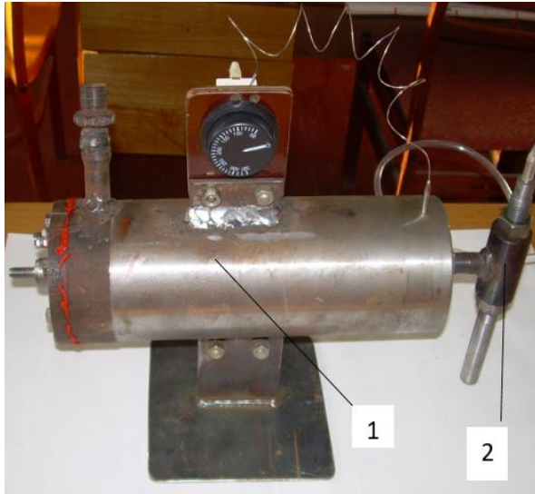
Fig. 3. Gas-dynamic spraying device. 1 - compressed air heater. 2 - nozzle accelerator of compressed air and spray powder.
