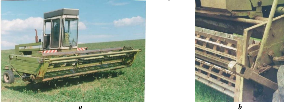
Fig. 2. General view of the E-303 (a) mower and flattening roller (b) Source: author's proposal
