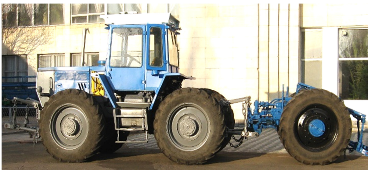
Fig. 3.3 – Modular power vehicle of traction class 3 – 5 on the basis of HTZ-160 tractors
