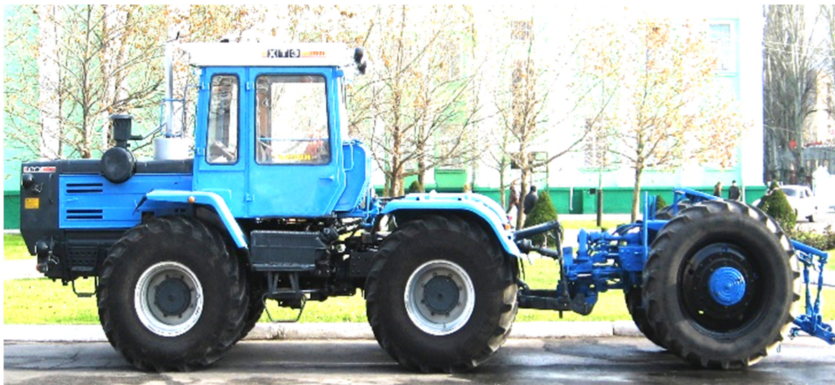
Fig. 3.2 – Modular power vehicle of traction class 3 – 5 on the basis of HTZ-170 tractors
