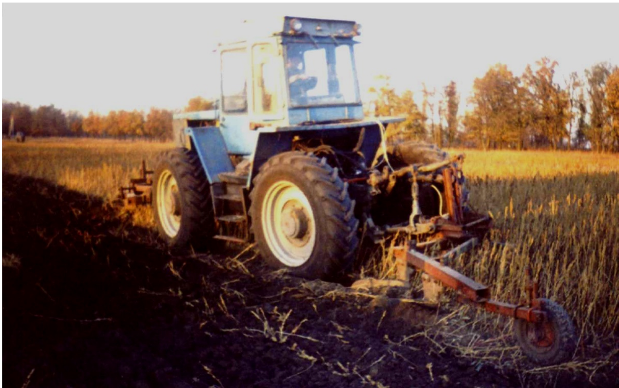
Fig. 2.27 – Wheeled tractor HTZ-120 in aggregate with rear-mounted four-bodied and frontal two-bodied plows during field experiments
