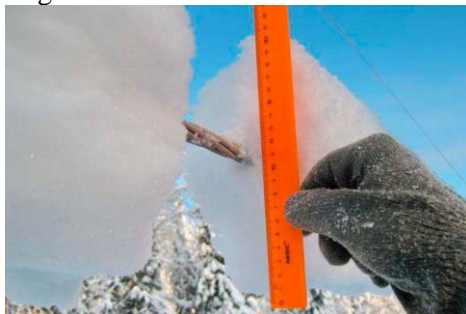
Fig. 2. Ice on the wire
