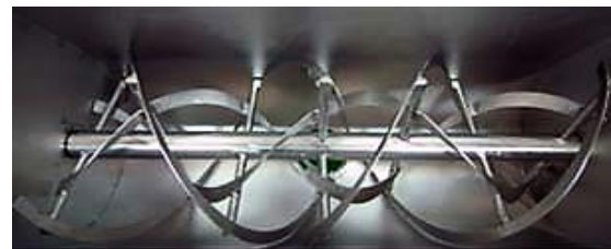
Fig. 8. Shaft with two "S" type belts
