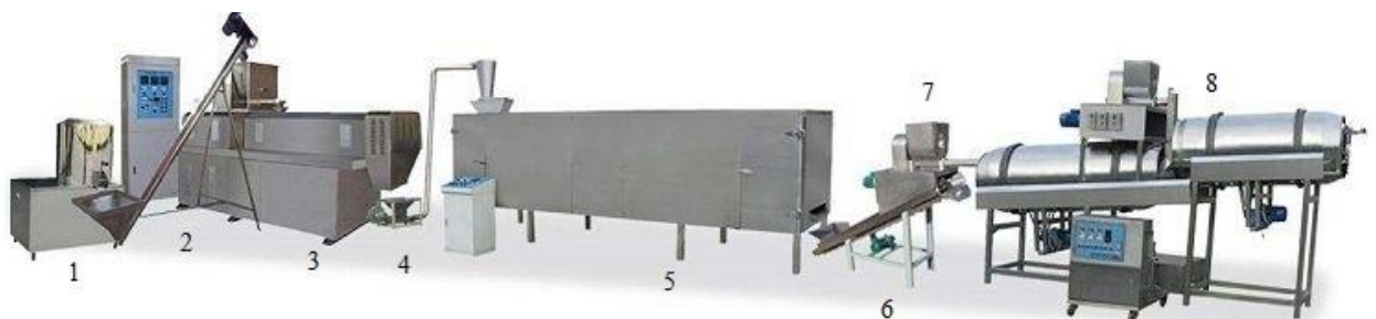
Fig. 4. Production line for corn snacks: 1 - mixer; 2 - screw conveyor; 3 - extruder; 4 - air conveyor; 5 - dryer; 6 - conveyor; 7 - sprayer; 8 - cooler
